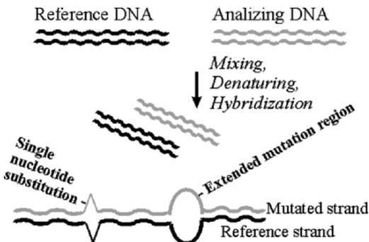
Figure 1. When hybridized to reference wild-type DNA, mutated DNAs form heteroduplexes with one or more mispaired nucleotides. These mismatch sites are targets for the majority of hybridization-based mutation detection techniques.
