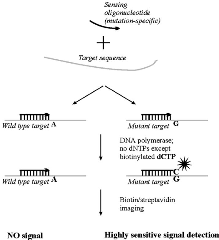
Figure 10. Schematic representation of the enzyme-amplified electronic transduction assay principle (see text).
