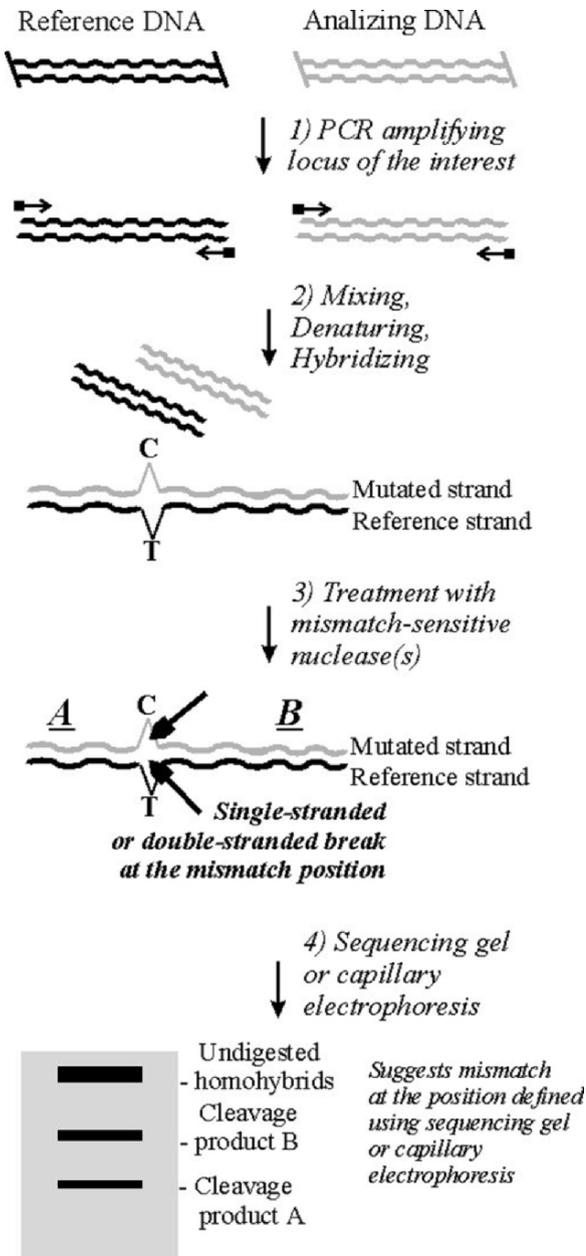
Figure 3. Generalized scheme for the enzymatic hybridization-based mutation detection approaches.
